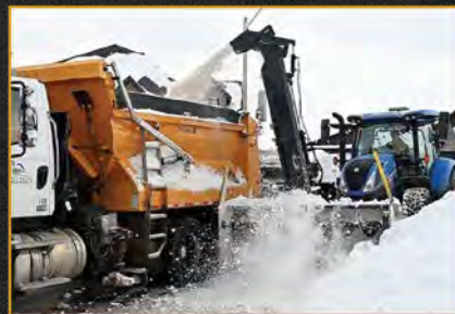
TRUCK LOADING CHUTE
