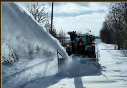
ROTATING FAN HOUSING / SIDE DISCHARGE
