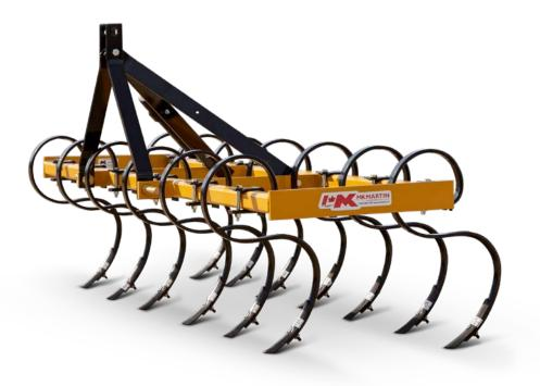
MK Martin **Cultivators** are the ideal tool to be used in small fields and gardens. Equipped with two rows of S-tines this cultivator provides thorough penetration aerating the soil and preparing seedbeds. Each tine features easy single bolt adjustment allowing you to adjust your soil distribution as required. Each S-tine also features replaceable bolt-on tips allowing for easy individual replacement as needed.
