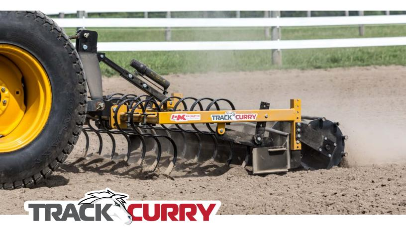
This easy to use tool will allow you to condition indoor or outdoor track surfaces that have been packed or compressed by heavy traffic or natural elements such as heavy rains, to restore your riding surfaces in a single pass.
