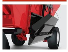
The optional center dump directs the unloading material beneath the gravity box, ideal for when the unloading area isn't wide enough for standard side dumping.
