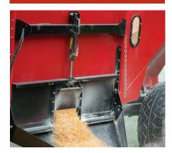
The optional Hydraulic Door allows you to conveniently control the metering of the material using a remote from your tractor.
