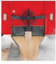
Each Gravity Box comes with an easy to use unloading door equipped with a metering door, providing a smoother, more consistent flow of material. It also allows you to fine tune the amount of material leaving the Gravity Box ensuring that you're in control of the flow every time.
