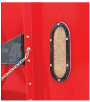
Conveniently located beside the unloading door, these viewing windows allow you to see the current level of material inside the Gravity Box.
